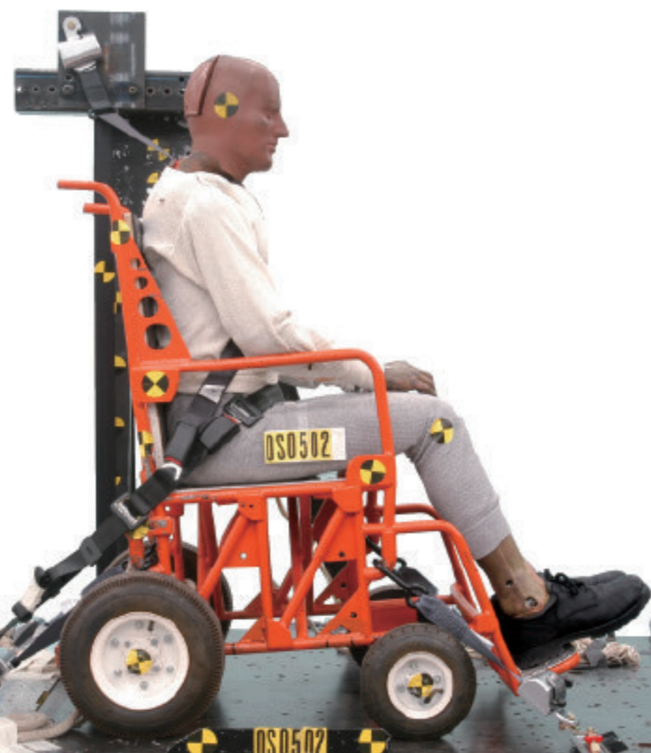
Kit: B-001 4 (ALR) Retractors with Lap Belt Pin Connector Quick-Connect Fitting 1 Lap Belt
